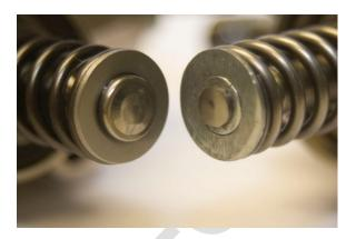
Upon further disassembly, you can see the wear that is taking place inside the pump. Here is a shot of the competitor's spring retainer. You can see that it has completely cracked and deformed under the pressure.
