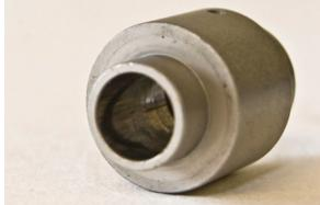
Finally, now that the shaft has been removed from the pump we can get a closer look as to how its 'eroded' over time. The face is no longer flat, and the sides are very sharp.
