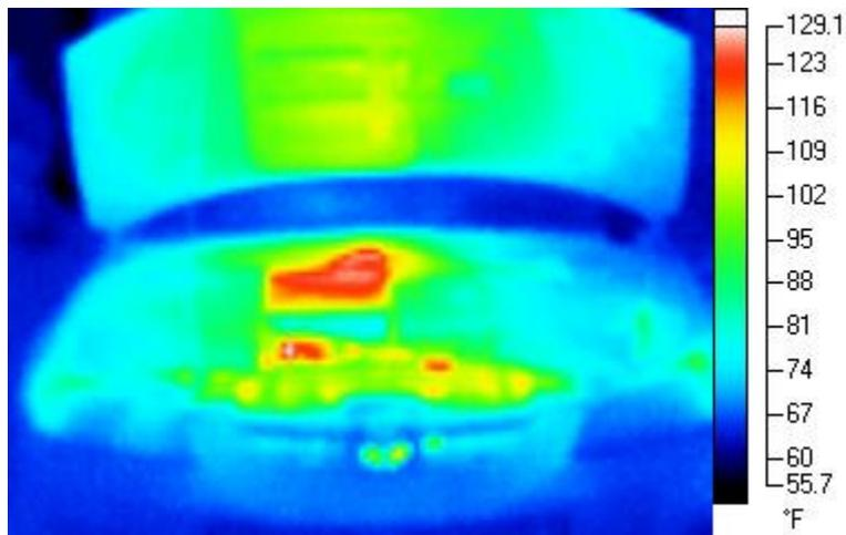
Since the cp-e™ intercooler is in front of the car, it will receive very little heat transfer. This is ideal as the intercooler is now only responsible for cooling the intake air, as opposed to waste heat from the engine. You can see the blue rectangle behind the bumper, which indicates a temperature of about 75°F.
