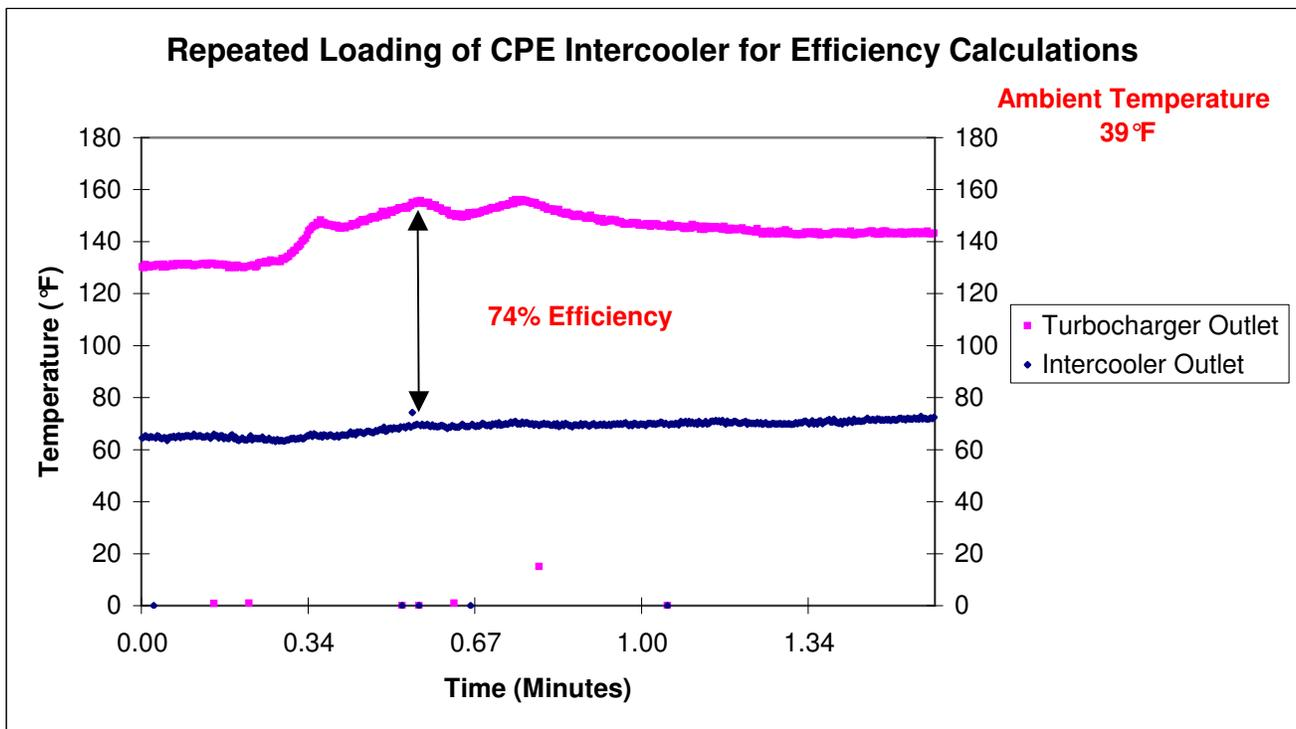
The cp-e™ intercooler found the fine balance between cooling efficiency and pressure loss. Because our core doesn't sap as much energy from the air, simply adding this core to a stock car would allow nearly a three-pound increase in boost pressure to the engine. Moreover, our intercooler is much more stable than the stock unit, as it is not as sensitive to heat input. You can beat the turbocharged MZR for all it's worth, and our intercooler will maintain its 70%+ efficiency rating.
