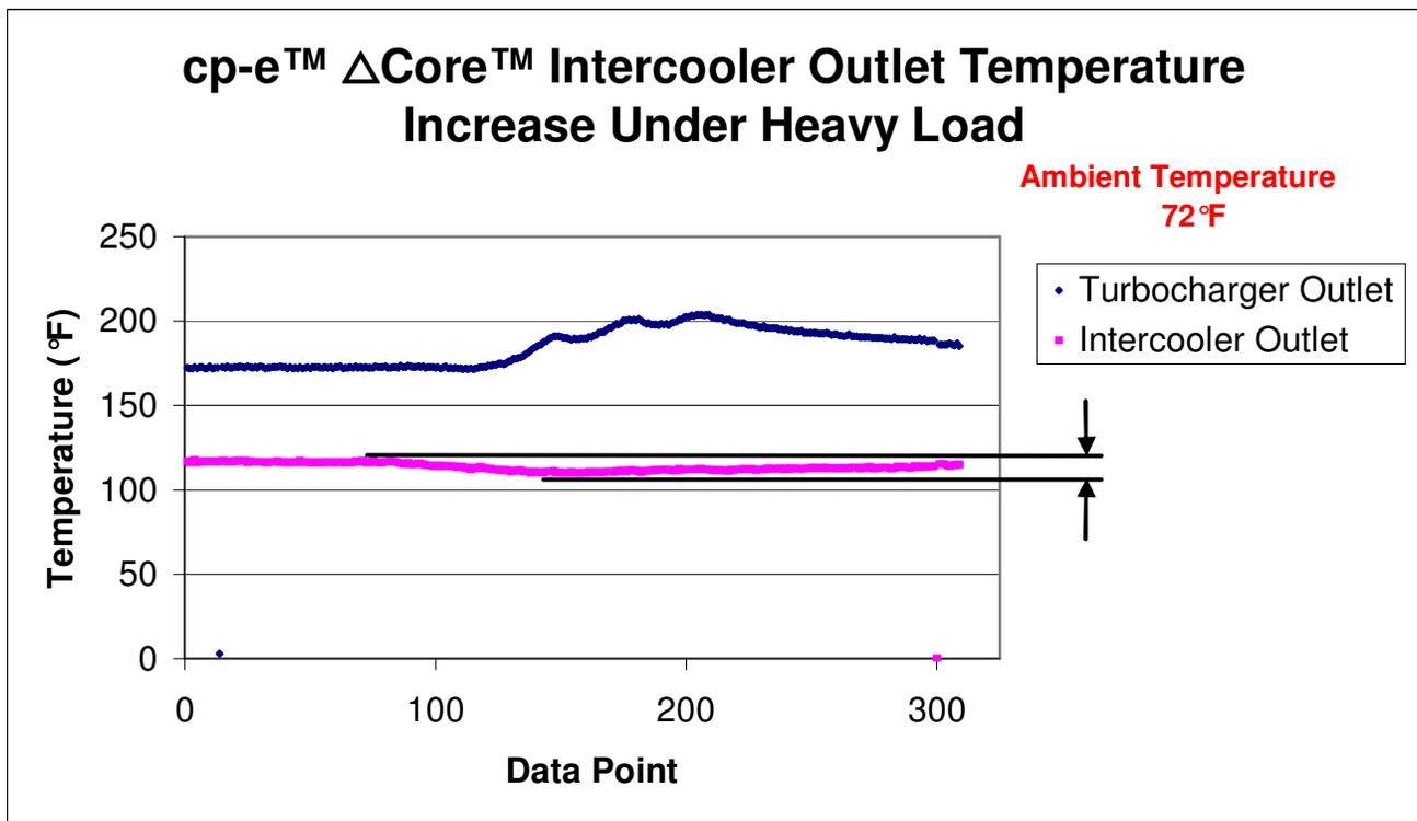
Notice the temperature increase of both the boosted air before and after the intercooler. Despite a 40°F increase in boosted air temperature, the temperature of the air exiting the cp-e™ intercooler is almost unchanged! In fact, the intercooler outlet temperature seems to *drop* once the throttle is pinned. This is probably due to the increase in air speed while the throttle was applied.
