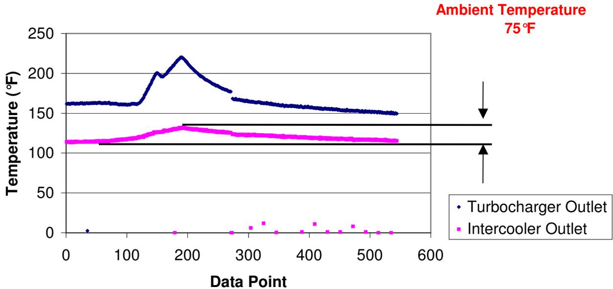
Notice how sharply the temperature of the air coming out of the intercooler increases under boost. Even though the boosted air is hotter than the cp-e™ example, the stock intercooler increases the outlet temperature by as much as 30°F! If we had been able to load the intercooler for longer than a few seconds, the problem would be even more apparent.
