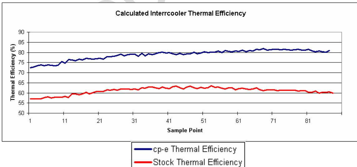
It comes as no surprise that the cp-e™  $\Delta$ Core™ intercooler has a higher efficiency than the stock intercooler considering that it managed a higher total temperature drop. A decent intercooler should have a thermal efficiency of about 65%, which the stock intercooler barely falls short of
